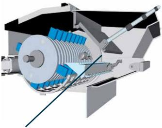
FlexRejectDoor™ This is a safety device which prtects the mill from damage and stoppages if any uncrushable material is fed in by mistake.
