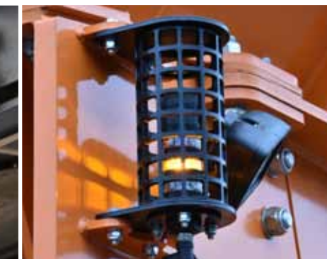
Machine operating mode indicator - for status check and security warnings
