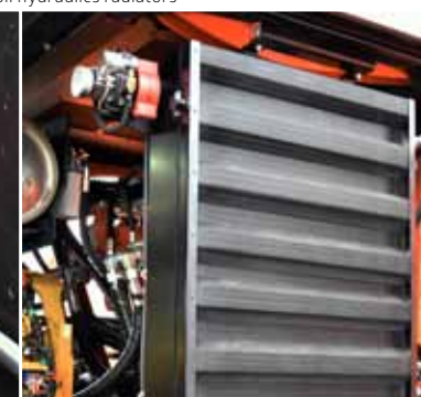
Cleanfix systems automatically clean engine and oil hydraulics radiators
