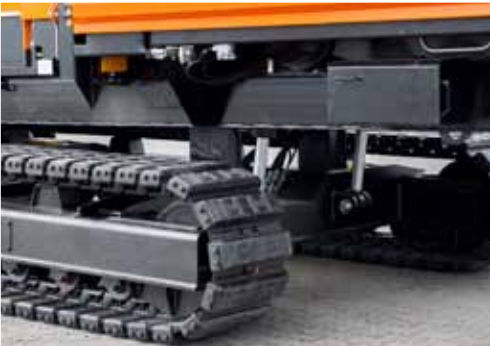
Hydraulic system for adjusting chassis position in MPB 20.55gh. The mechanism allows leveling machine on longitudinal slopes and increases the clearance for easier moving on uneven terrain
