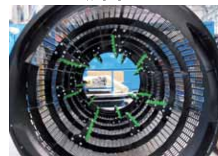
Screwed knives for ripping bags with waste*
