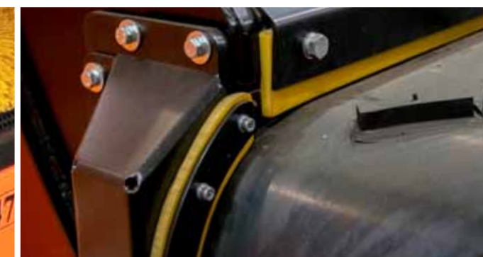
Sealing in the hopper prevents material from leaking to the inside of the machine
