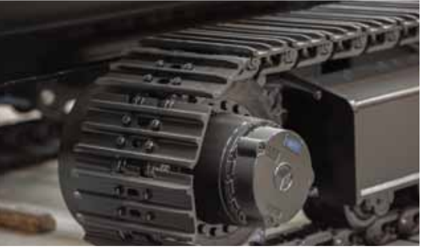
Tracked chassis for moving the machine without any additional towing vehicles
