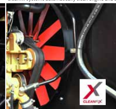
Cleanfix systems automatically clean engine and oil hydraulics radiators
