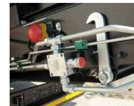
Belt speed adjustment - adjusts the speed to the type of screened material to maximize the performance. It also allows to stack more material of each fraction without the need of re-locating the machine
