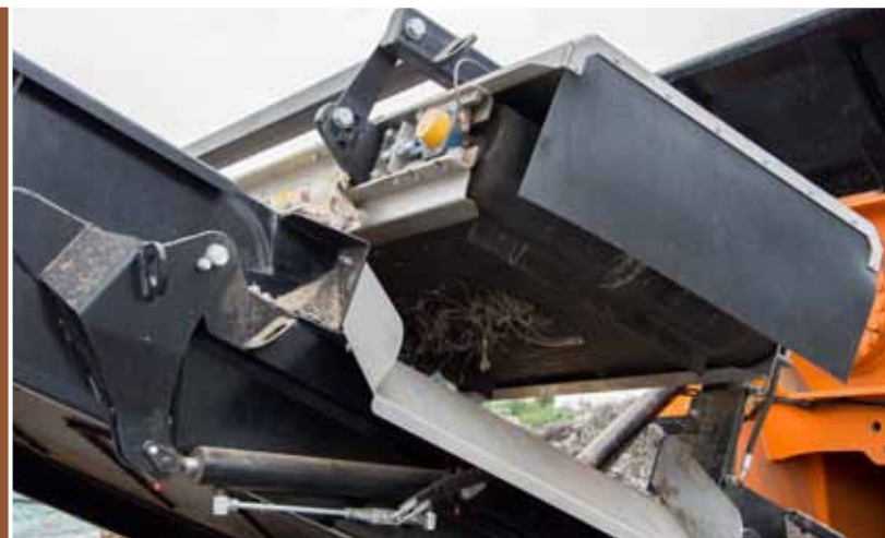
Magnetic separator for extraction of ferromagnetic materials.
