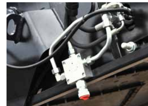
Conveyor belt speed rate adjustment
