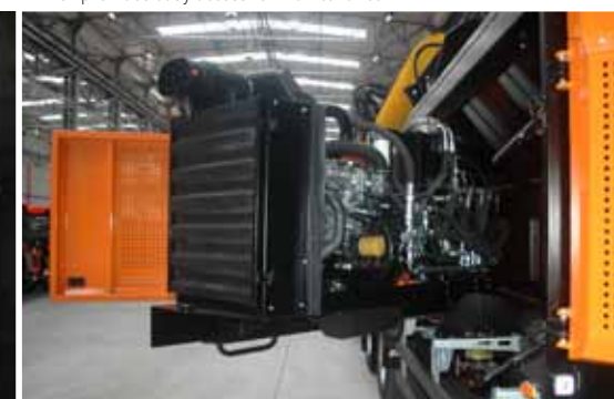
The engine and hydraulic system are mounted on a pull-out frame which provides easy access for maintenance
