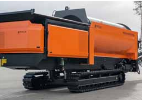
Hydraulic system for adjusting chassis position in MPB 20.55gh. The mechanism allows leveling machine on longitudinal slopes and increases the clearance for easier moving on uneven terrain
